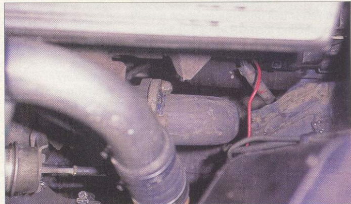
11 The exhaust down-pipe was refabricated with a new manifold flange and a tighter bend, to avoid fouling the bulkhead
