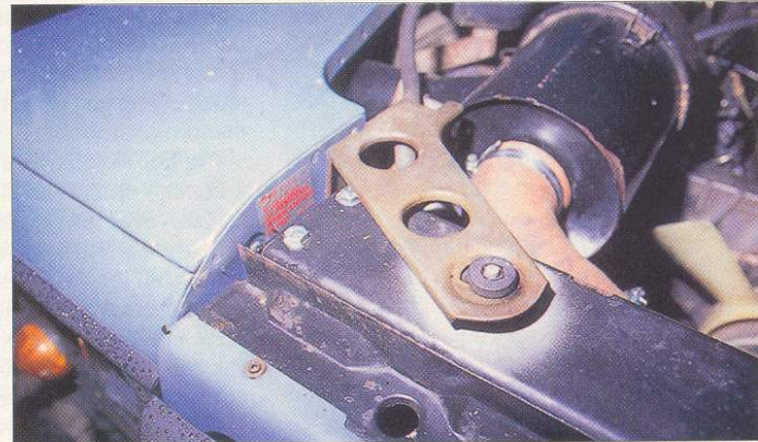
12 Radiator mounting spigots were transferred to the top of the casing to match the 90 brackets on the inner wings
