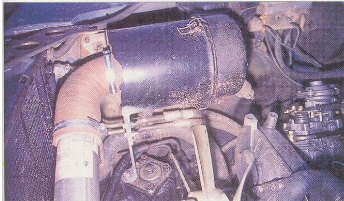
5 To make more space for the turbo outlet pipe, the air filter was re-sited on the right-hand inner wing, using specially-made brackets
