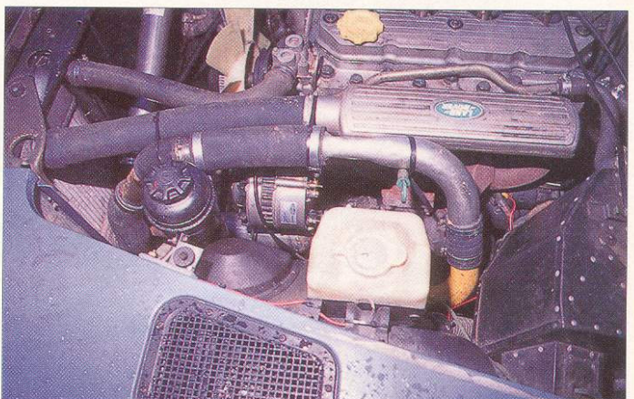
4 Main piping problems centred around the turbo air connections. Steel pipe has since been painted black to prevent rusting
